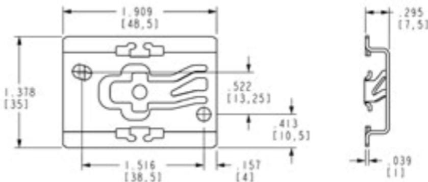
NOTE: The XMD is compatible with standard 35mm DIN Rail with 1 mm thickness. Use the bracket dimensions to source the proper DIN Rail size.
